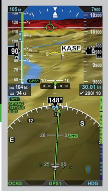
Evolution Synthetic Vision (ESV) is an optional expansion to the Evolution Flight Display System. ESV presents a real-time, computer-generated 3D view of terrain, obstacles, and traffic.
